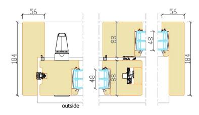
Sash width 756 ... 2045 mm Sash height 646 ... 2545 mm Sash weight up to 200 kg Sash height: Sash width = max 2:1 Jamb width 1500 ... 6400 mm Jamb height 750 ... 2650 mm
